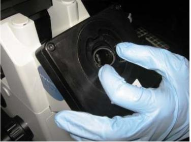
**Removing the Polarizer from the Eyepiece Filter Wheel** Leave the white Eyepiece assembly off for now.
