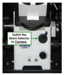
Acquire images continuously (**File** | **Continuous Acquire**) as you rotate the knob on the Principal Prism Slider to adjust the contrast displayed in the images. For example, move the shadows from bottom to top and move the black line into or out of the image.
